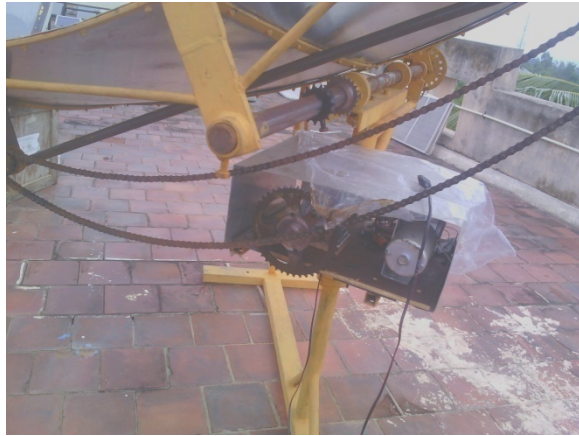
Fig. 3: Working of tracking set up for the concentrator
